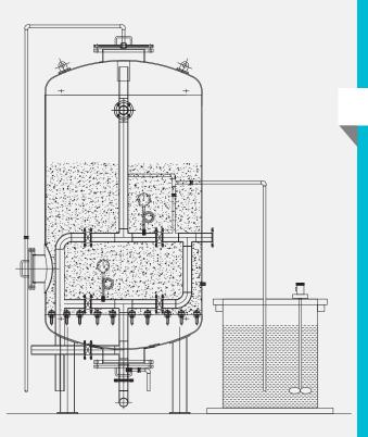
Water Softener is used to remove minerals such as calcium, magnesium, and certain other metal captions in hard water. Reducing the tendency of scale being formed in equipment such as Boiler, pipelines, and engine jackets.
