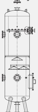
**Vacuum Dryers** are used for the drying of palm oil under vacuum before sending it to the CPO storage tank.
