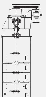
**Fruit Digester** come with intermediate shaft for long operational life of parts, easy alignment and easy maintenance.
